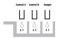
Always use a new pipette for each sample or standard. Keeping the pipette vertical, add:
